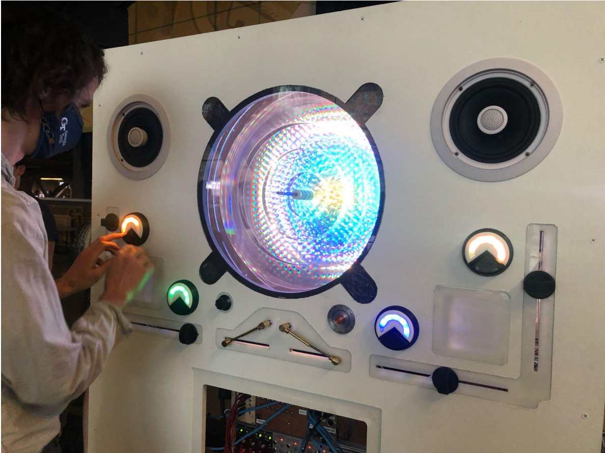
Figure 8. Demonstration of the instrument at the Expo. Notice how the 4 button lights correspond to sliders and to different rings of light inside the visual display.
